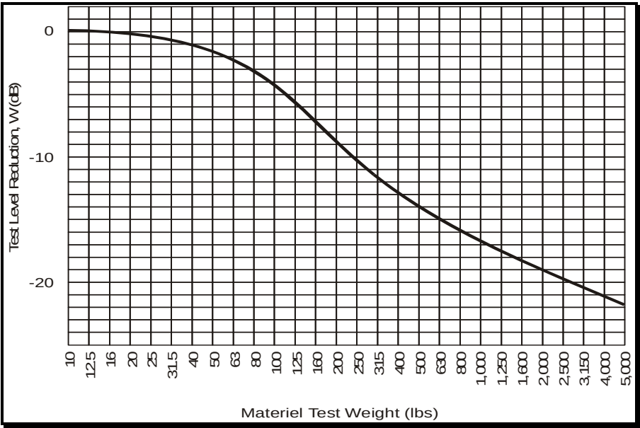
FIGURE 519.6D-5. Test level reduction due to materiel mass loading.
