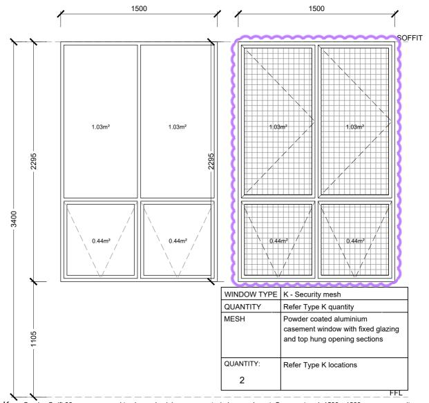
Type. K Crealco Swift 38 or eq. approved top hung aluminium casement window, per layout. Casement sash 1500 x 1200mm max capacity
