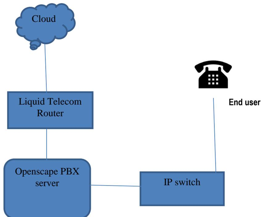
The current setup does not need any internet connection. We use liquid telecoms router to connect to the outside world to make and receive external calls.
