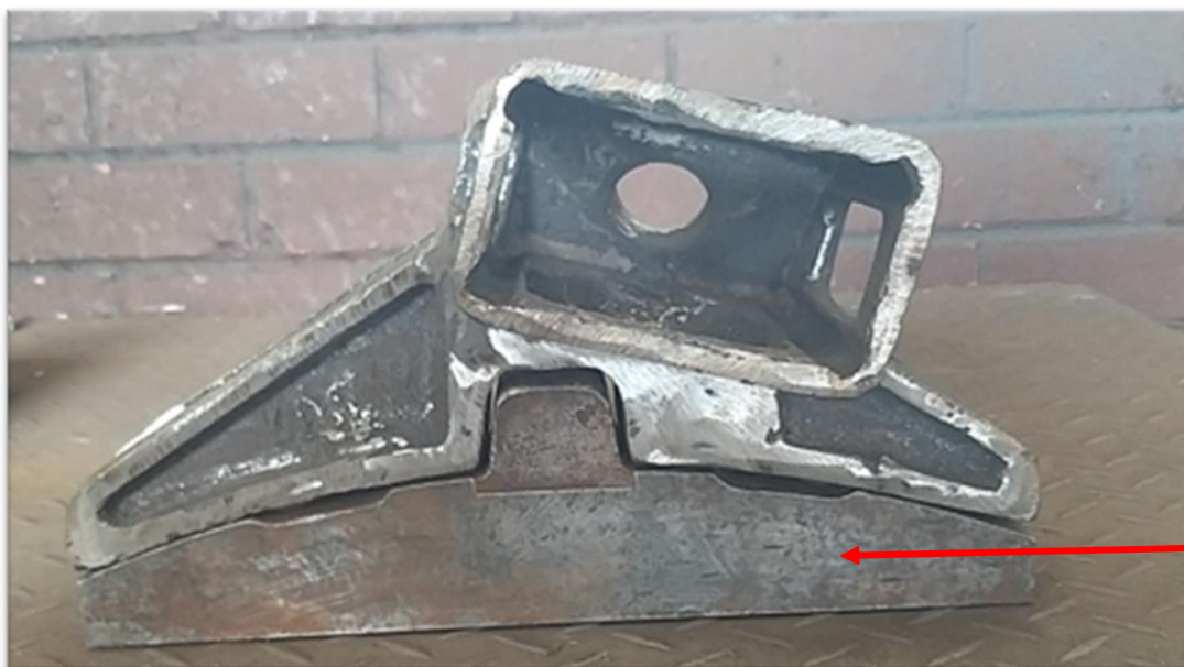
Figure 9: Illustrates the actual first gauging of the Brake shoe.
