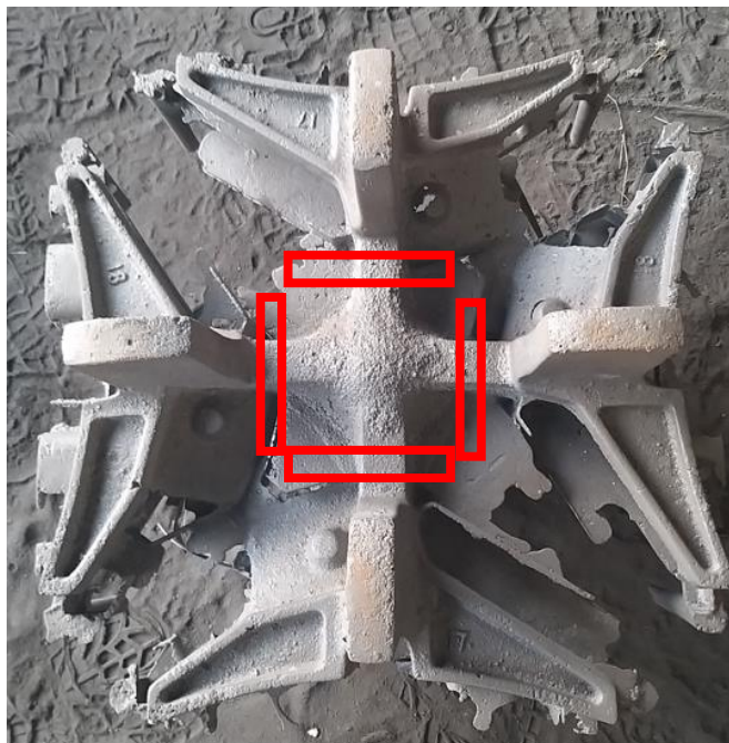
Figure 3: Illustrates a bottom view of brake shoe and relevant sections to be cut off. (NB: Removal of flesh is necessary)
