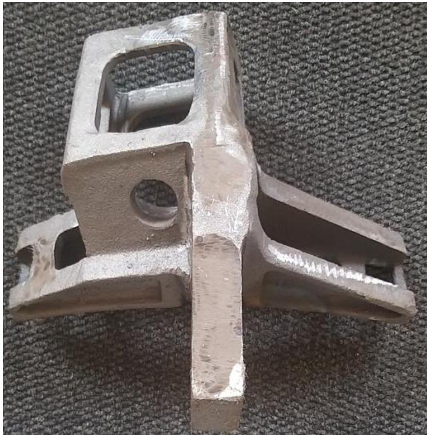
Figure 6: Illustrates a typical KDS Foundry Brake shoe post fettling.
