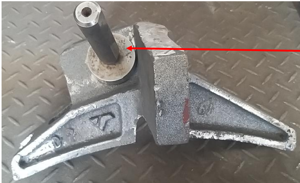
Figure 11: Illustrates the third gauging of the Brake shoe.
