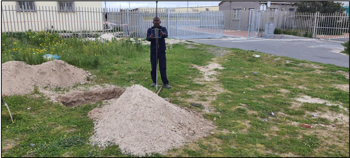
Figure 5: DCP testing conducted on site.
