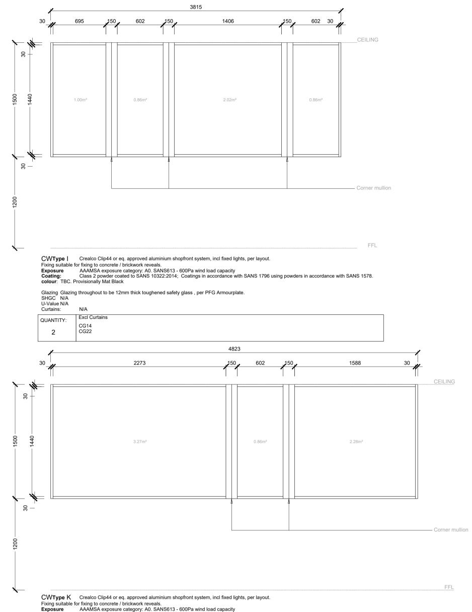
Class 2 powder coated to SANS 10322:2014; Coatings in accordance with SANS 1796 using powders in accordance with SANS 1578.
