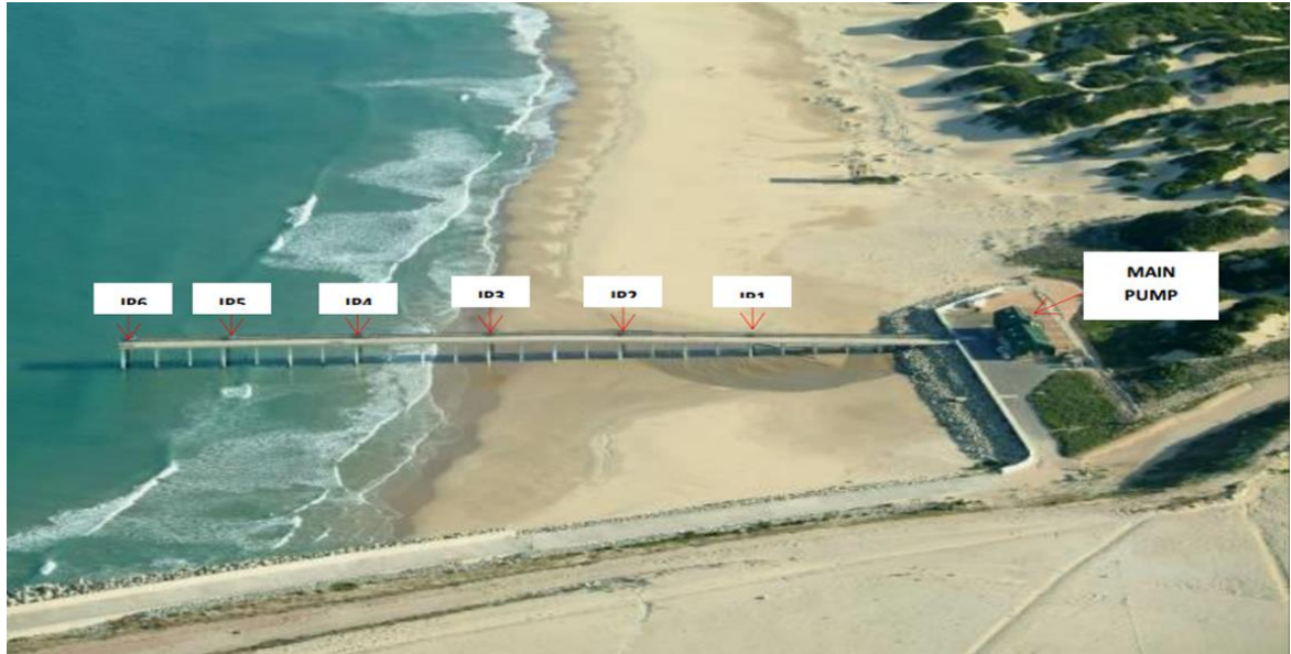
Aerial view of Sand Bypass Jetty, showing the full length of pipeline including all Jet pumps (JP1 to JP6)
