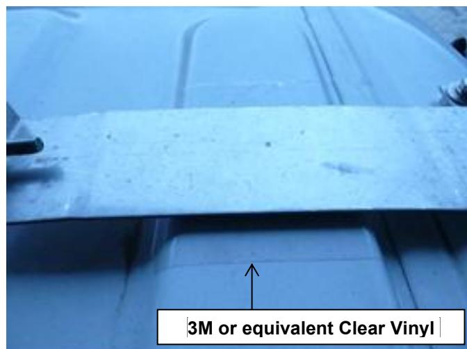
3M or equivalent Clear Vinyl (Paint Protection Film) between the bracket and the paintwork of the vehicle
