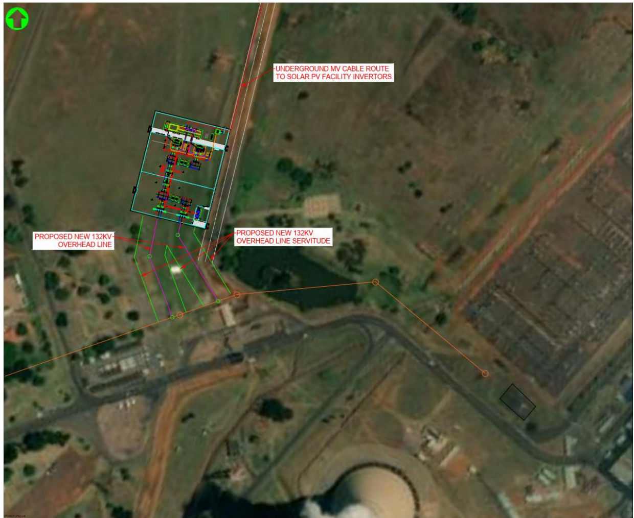
Figure 6: Proposed Loop in Loop out layout
