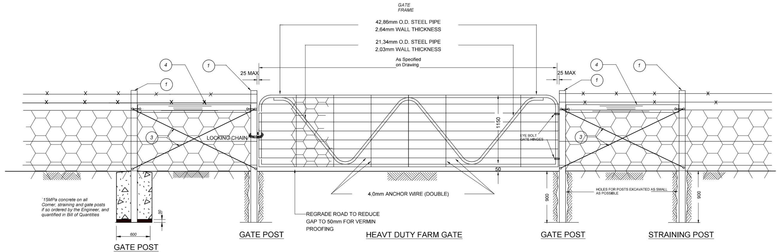
\*15MPa concrete on all Corner, straining and gate posts if so ordered by the Engineer, and quantified in Bill of Quantities
