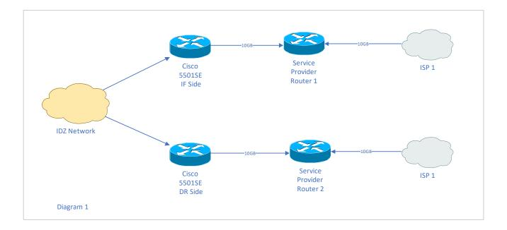
We are currently consuming 2Gb service and have redundant fiber routes to both our datacenters. These links are currently connected with 10Gbps fiber modules (LC factor) with single mode fiber. Both Datacenters have Uninterrupted Power Supply (UPS) and backup generators.
