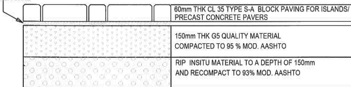
TYPICAL BRICK PAVING/ PRECAST CONCTETE PAVING LAYERWORK DETAILS N.T.S
