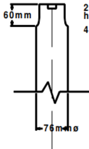
Drawing 11 - 76mm pole top details
