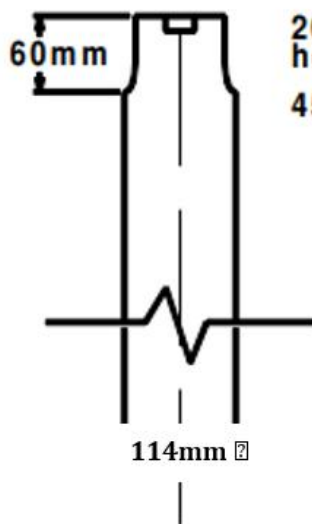
Drawing 12 - 114mm pole top details
