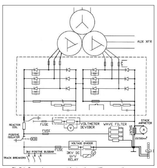
Fig 7.1: General arrangement for traction rectifier connections.
