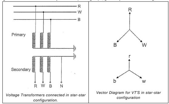
With this arrangement the secondary voltages provide a complete replica of the primary voltages and any voltage (phase-to-phase or phase-to-earth) may be selected.
