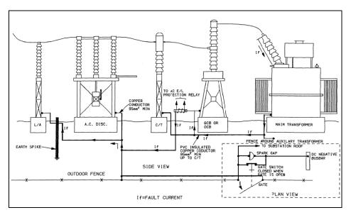
Figure 9.1:Typical AC Earth leakage protection systems.
