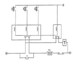
IDMTL Overcurrent + Time Lag Earth Fault
