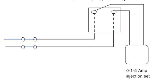
Figure 15:3 Connections for testing AC Ammeter.
