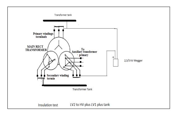
Figure 5.4: Insulation test LV 2 to HV & LV 1 & Earth
