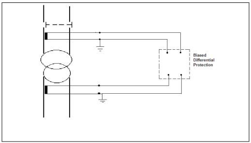
Figure 14.3: AC Substation General Arrangement for Main Transformer Biased
