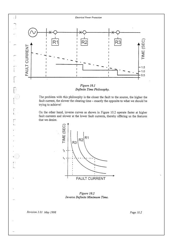
With modern programmable relays IDMT Curves applicable to electromechanical relays can easily be obtained from the wide range of curves available.
