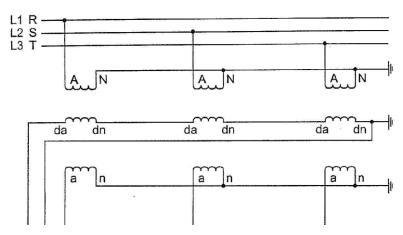
A set of VT's with one Y-connected and one broken delta secondary circuit.
