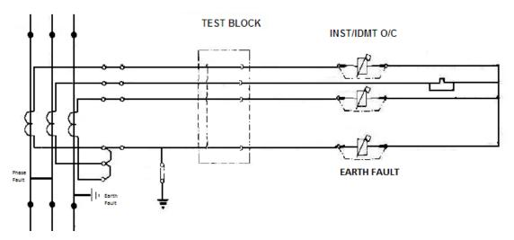
Fig 20.4 Typical connections for general O/C and E/F protection
