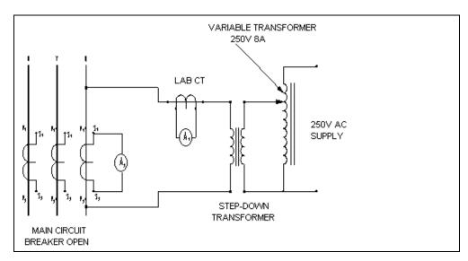
Figure 4.6: Test Circuit for Current Transformer Ratio test
