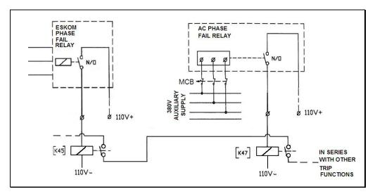
Figure 21.1: VT supply from Eskom VT utilised for "AC Fail/Available" with alternative from auxiliary supply.
