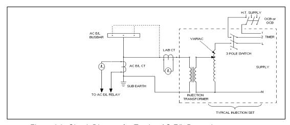
Figure 6.2: Circuit Diagram for Testing AC E/L Protection
