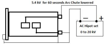
Figure 18.1 Hipot insulation test
