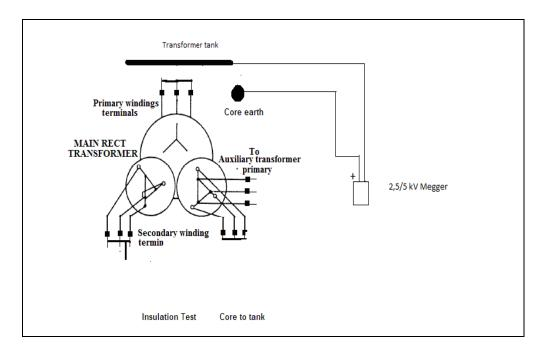
Figure 5.5 Insulation test Core to tank
