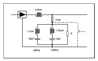
Fig 12.2 12<sup>th</sup> and 24<sup>th</sup> harmonic filter for a 12 pulse rectifier
