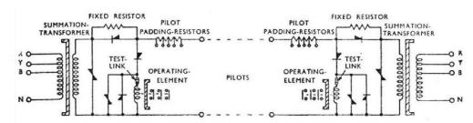
Fig.X.6.-Schematic diagram of complete "Solkor-R" protective system
