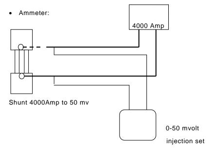
Figure 15:1 Connections for testing DC Kilo Ammeter.
