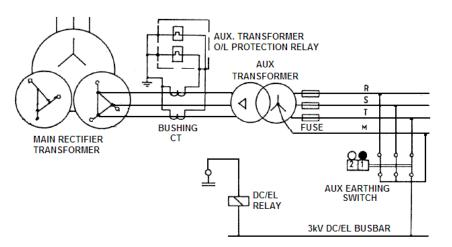
Figure 9.1: Typical connection for Auxiliary Transformer as arranged in Traction substations.
