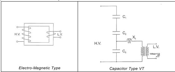
The magnetic voltage transformer is similar to a power transformer and differs only in so far as a different emphasis is placed on cooling, insulating and mechanical aspects.
