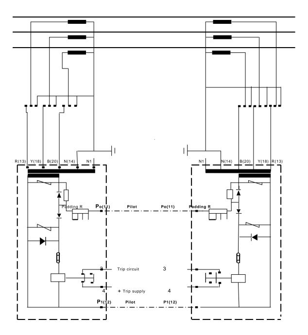
Figure 20:9:Typical schematic diagram for a SOLKOR feeder protection system.
