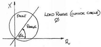
Changing the settings of the relay will change the size of the circle, the position of the mid point of the circle (as determined by the phase angle  $\Phi$ ) and also the time delay before tripping the VCB.
