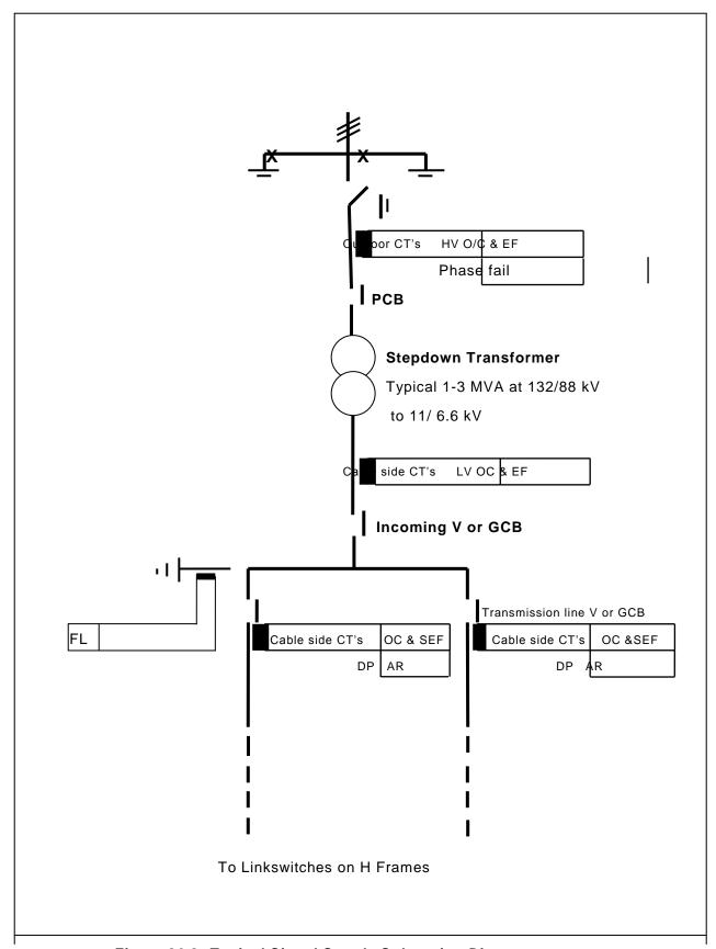
Figure 20.2: Typical Signal Supply Substation Diagram
