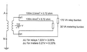
The accuracy of a Voltage Transformer is guaranteed at the Secondary Terminals.
