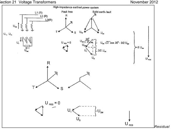
Voltage (neutral displacement voltage) from an open Delta Circuit
