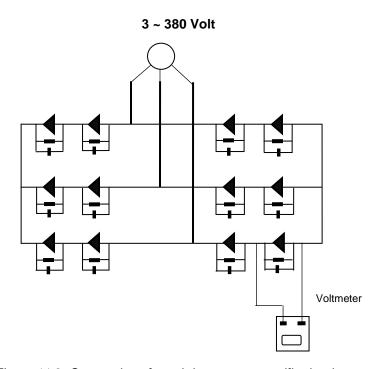
Figure 11.2: Connections for voltdrop test on rectifier bank
