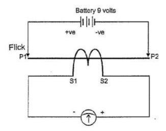
Connect centre zero galvanometer across secondary of the current transformer. Connect battery negative terminal to the current transformer P2 primary terminal. Touch or flick the positive battery connection to the current transformer P1 primary terminal. If the polarity of the current transformer is correct the galvanometer should flick in the positive direction.
