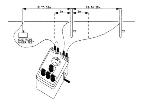
Figure 14.7: Connections for testing resistance between spike under test the current and potential spikes.
