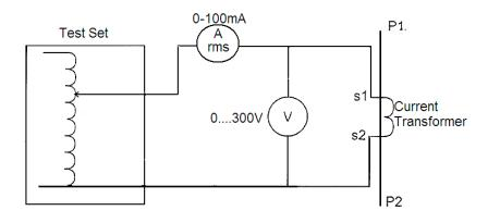
Magnetising curve test circuit
