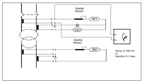
Figure 14.3: Connections for secondary injection
