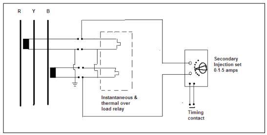
Figure 8.2: Connections for secondary injection test
