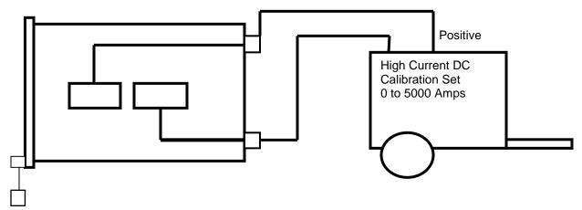
Figure 18.2 Circuit for Calibration of HSCB
