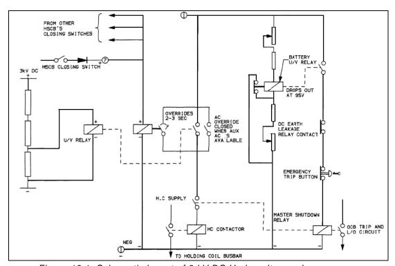
Figure 16.1: Schematic layout of 3 kV DC Undervoltage relay
