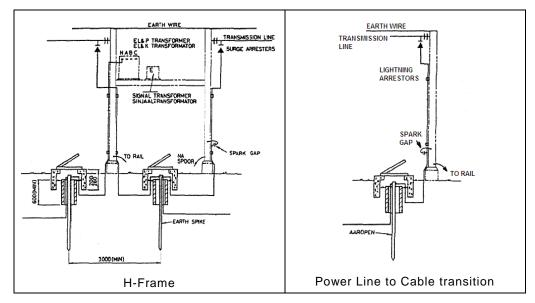
Figure 14.5: Typical H Frame stepdown point earthing arrangement
