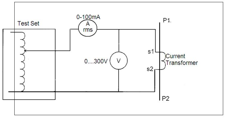
Figure 4.7: Connections for Magnetisation curve test.
