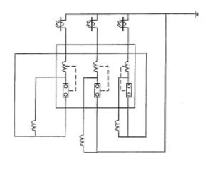
IDMTL OC+EF Relay with A C Trip Coils.
