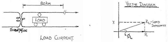
It can be seen that although  $Z_L\cong Z_F$ , the phase angles  $\Phi_F$  and  $\Phi_L$  are not equal:  $\Phi_F > \Phi_L$ . The YTG relay uses this difference to distinguish whether the current fed into the section is load current or fault current.
