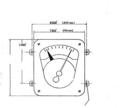
ler Model A131 which is being manufactured by Accurate Controls Ltd., Heath Works, Fordbridge Road, Sunbury-on-Thames, is designed for the protection of power transformers. The instrument is fully compensated for ambient temperature changes on capillary lines and case and operates in the following
