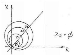
Each zone can then be used to protect up to the next VCB (although the relays are not normally set like this).
