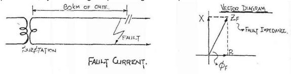
The impedance of the OHTE is highly reactive on a short circuit while the load drawn by a locomotive is mainly resistive (or closer to unity power factor).
