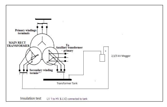
Figure 5.3: Insulation test LV1 to HV & LV 2 & Earth
