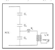
Primary voltages can range from 132, 88, 66, 33, 22, 11 and 6.6 kV with secondary normally at 110v. Protection of VT's is normally HV and LV fuses.
