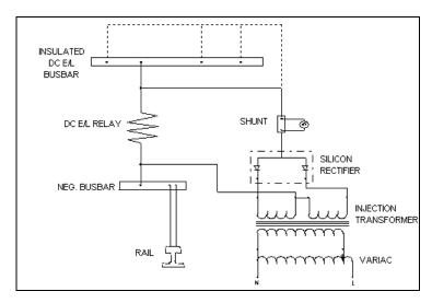
Figure 9.2: Circuit Diagram for Testing DC E/L Protection
