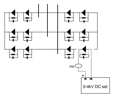
Figure 11.3: Connections for Peak Inverse Voltage test.
