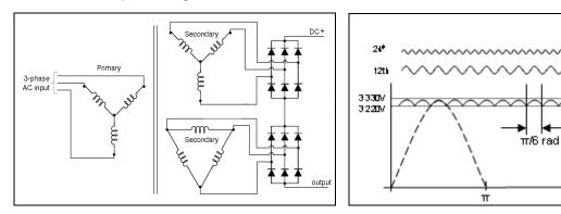
Fig 8.1: 12 pulse rectifier and ripple waveforms
