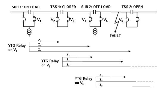
With a fault as shown, the YTG relay at  $V_5$  will see the fault as a  $Z_1$  fault, and trip immediately. If it fails to trip, the YTG relay at  $V_3$  will see it as a  $Z_2$  fault, and trip  $V_3$  after a time delay. The  $V_3$  relay will therefore act as back up protection for the  $V_5$  relay, the  $V_1$  relay as back up for the  $V_3$  and the  $V_5$  relay, etc.
