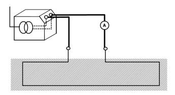
Figure 14:9 Earth connection tests
