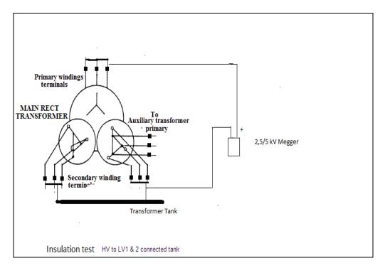
Figure 5.2: Insulation test HV to LV 1 & 2 & Earth
