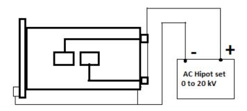
Test 2: HV Circuit Positive to HV Circuit Negative, frame and auxilliary circuits.
