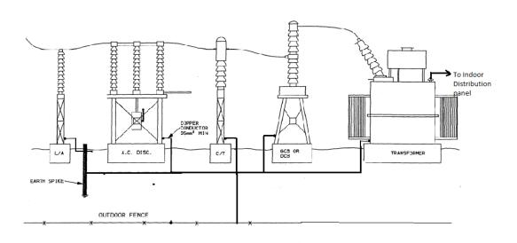
Figure 20.1: Signal Supply Substation outdoor yard layout
