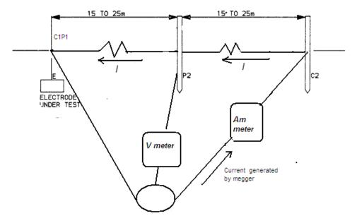
Figure 14.8: Equivalent circuit of earth test procedure.
