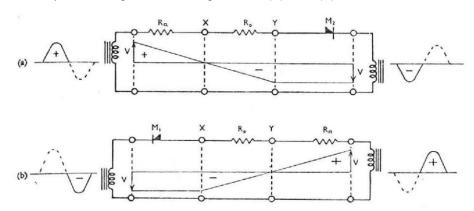
Fig.X.2.-Behaviour of basic circuit under external fault conditions.(a) and (b) show effective circuits during alternate half-cycle.
