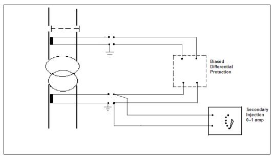
Figure 14.4: Connections for secondary injection
