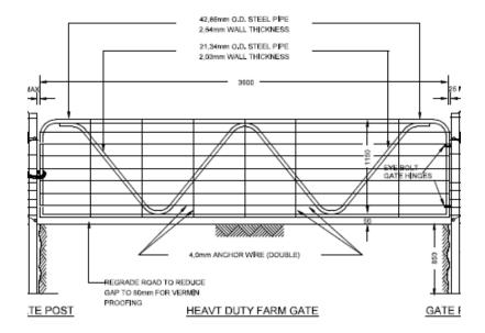
The frame shall be of tubing of bore 42 mm and wall thickness of 2,0 mm in the case of main frame members, and of a bore 22 mm and wall thickness of 2,0 mm in the case of bracing members. The width of each gate shall be as shown on the drawings.
