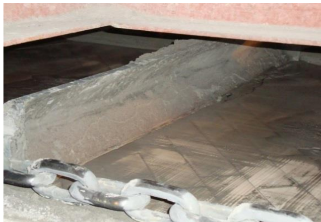
Figure 3: V shaped scraper bars running on a dry return trough.
