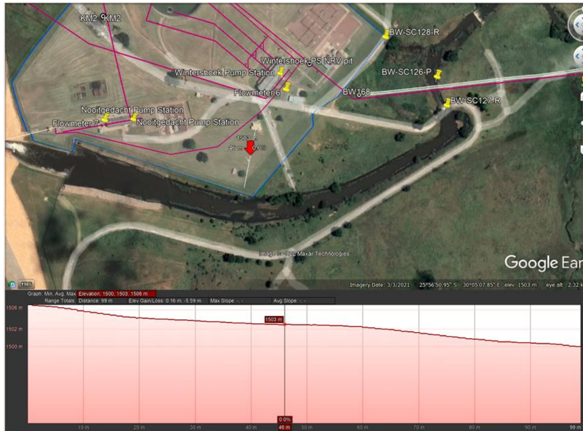
Figure 3: Wintershoek image showing elevations of flow from the ablution facilities to the existing sewage plant.
