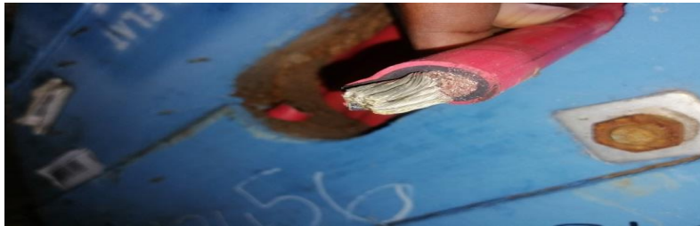
Fig 3 – Single core, 50 mm 2 red loco electric cable
