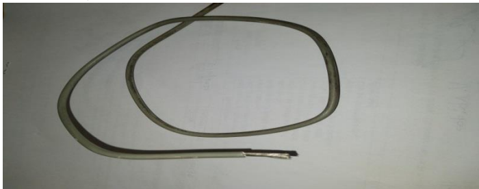
Fig 6 – Single core, 2.5 mm 2 light grey electric cable
