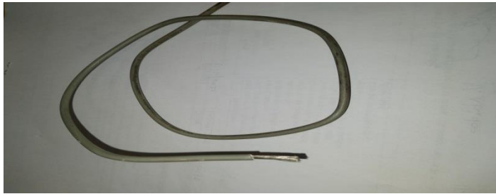
Fig 9 – Single core, 0.5 mm 2 light grey electric cable
