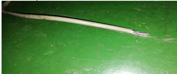
Fig 7 – Single core, 25 mm 2 light grey electric cable
