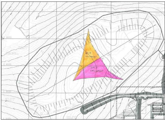
Figure 3: Temporary Clean Water Drain Catchment Areas
