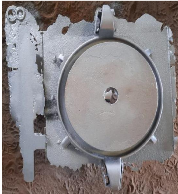
Figure 1: Illustrates the bottom view of a typical Bogie Centre as and when received by supplier.
