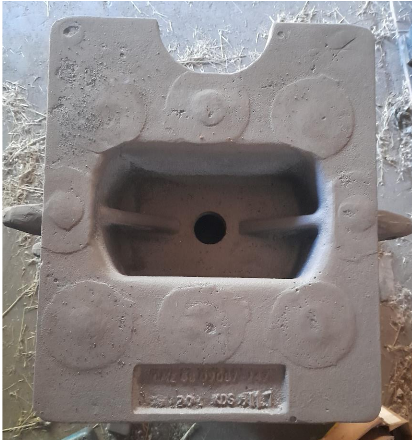
Figure 5: Illustrates the Bogie Centre expectations post cutting.
