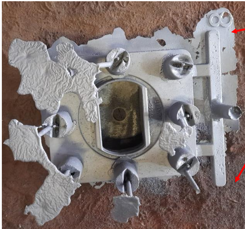
Figure 3: Illustrates the areas and sections to be cut off by Supplier.
