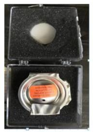
Used to protect against the trapping and possible over – pressurisation. It ruptures at 18 Bar.
