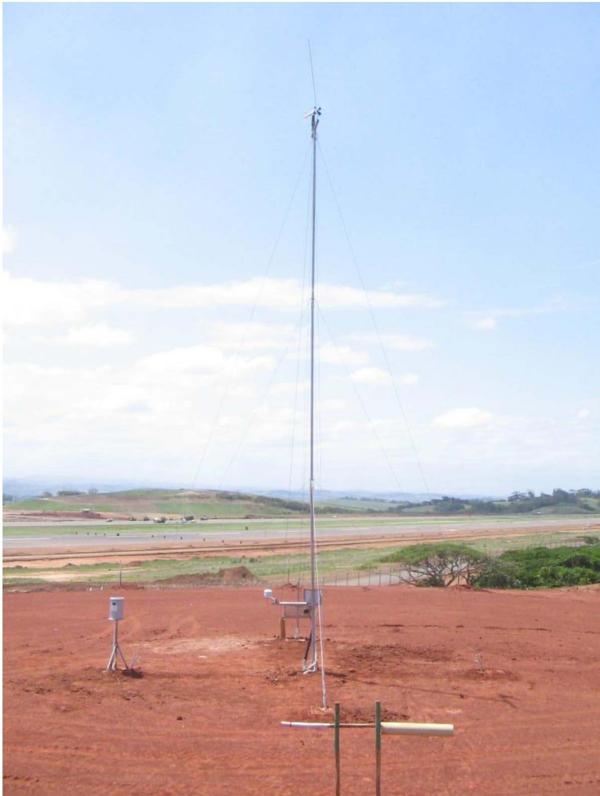
Picture of Automatic Weather Station (AWS) with raiguage to the left.
