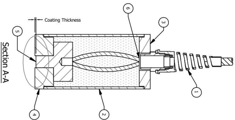
AC Monitoring Coupon 1cm<sup>2</sup> ø11mm
