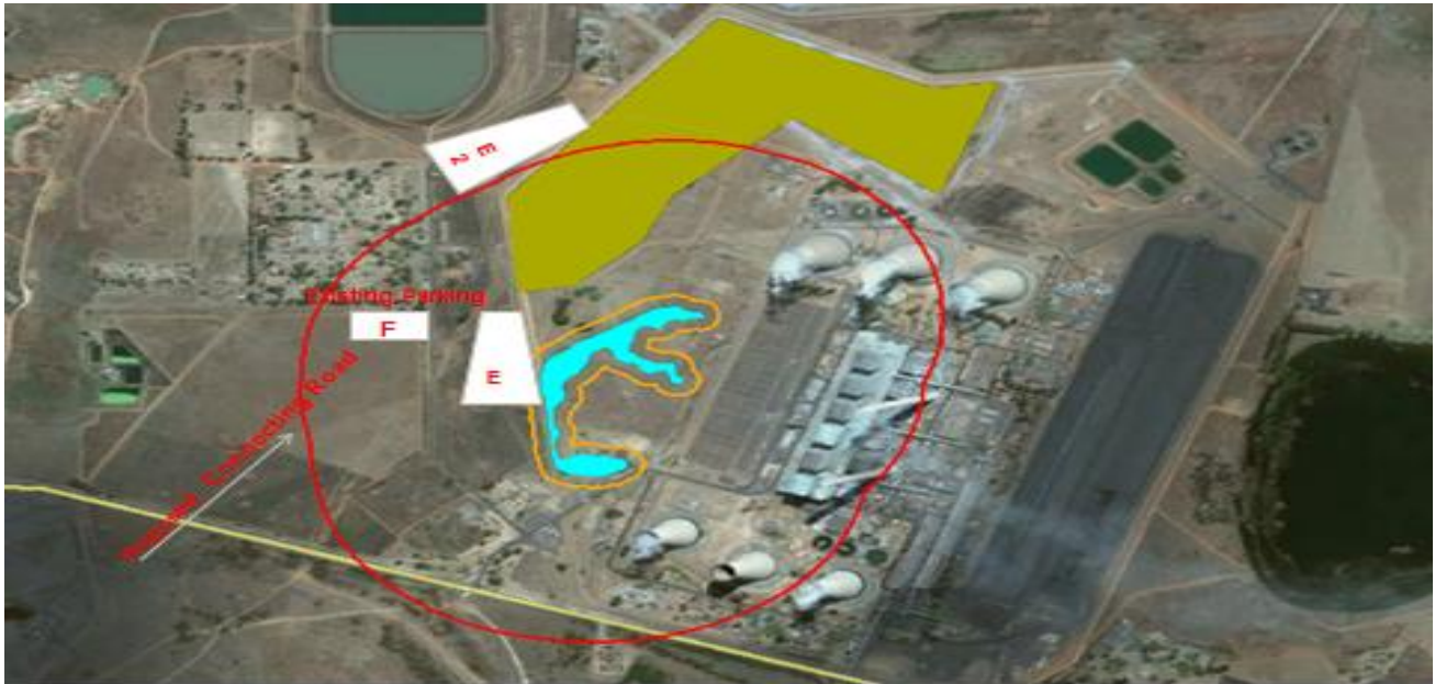
Area E: Originally Proposed Fabrication Area Area E2: Alternative Fabrication Area (Area E2 selected as suitable option) Access Road: Proposed one way connecting road to Area E2 (Traffic Management)
