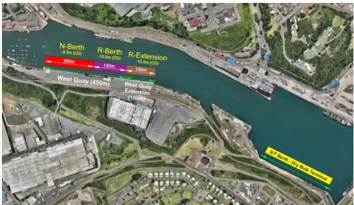
Figure 1: Orientation of the Port of East London Car Terminal Berths
