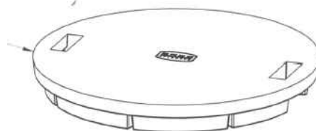
COMPONENT 3: CONCRETE INFILL
