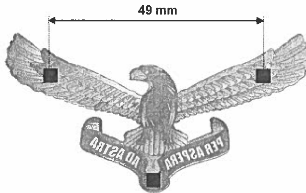
Figure 18 - Positioning of brass strips on cap badge (Item F)
