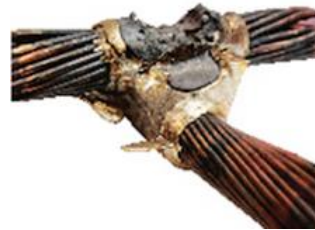
(b) Weld with excessive slag
