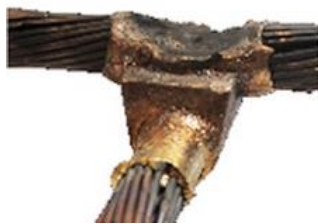
(a) Weld with insufficient volume to cover conductors
