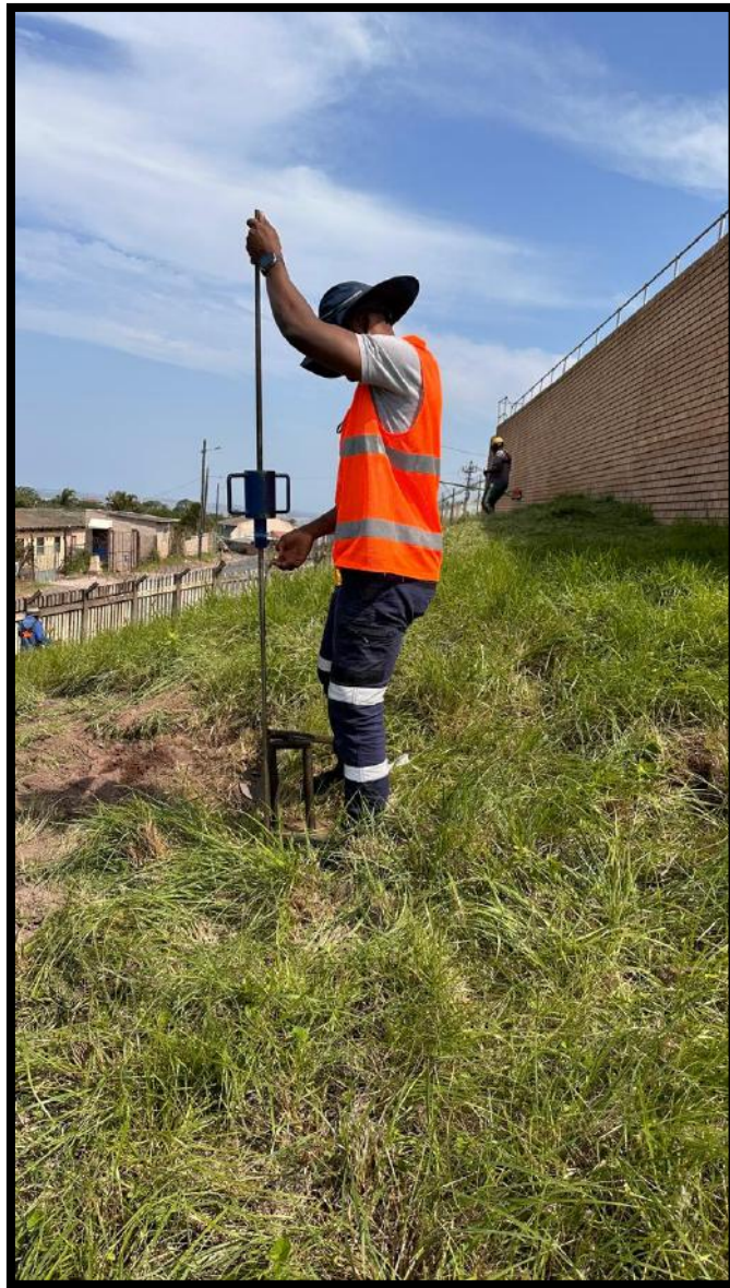
Figure 10: Showing the DCP testing undertaken at the site.
