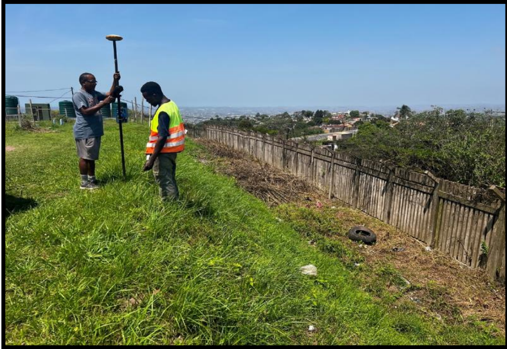
Figure 7: Showing the surveyor marking borehole positions at the site.
