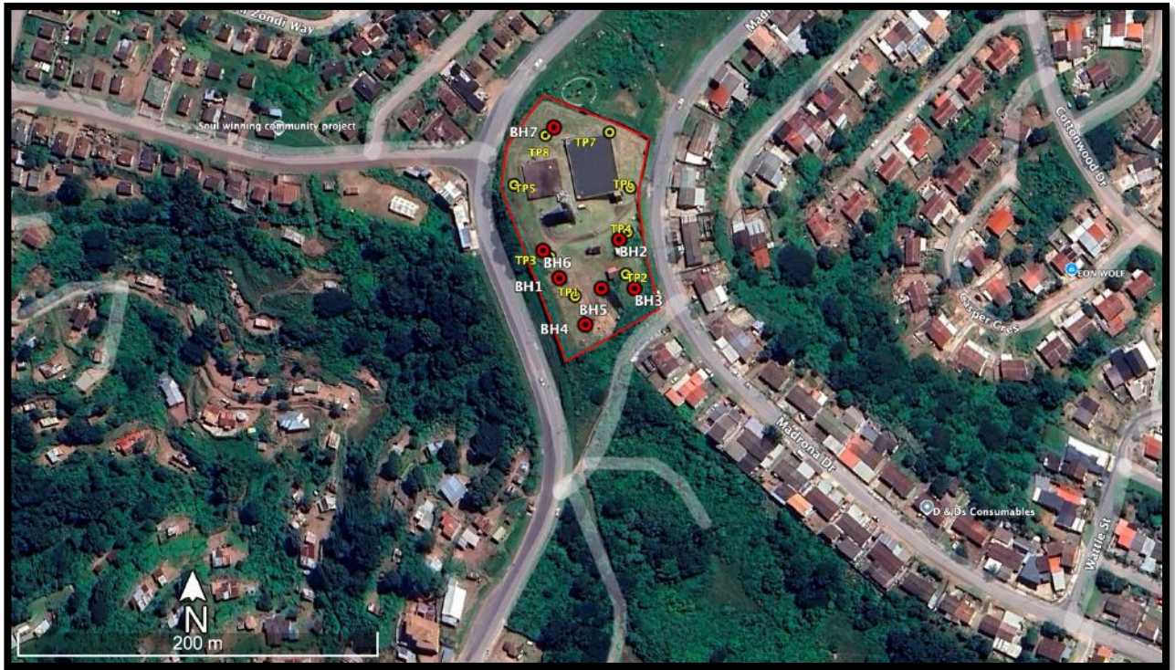
Figure 9: Showing the test pit (red dots) and borehole (yellow dots) position at the site.
