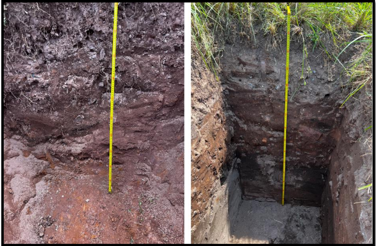
Figure 11: Showing the fill, transported, residual material, and sandstone exposed in the test pit at the site.
