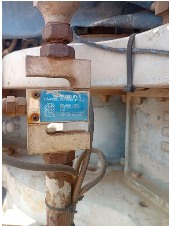
Figure 5: Pitch Moment Measuring
