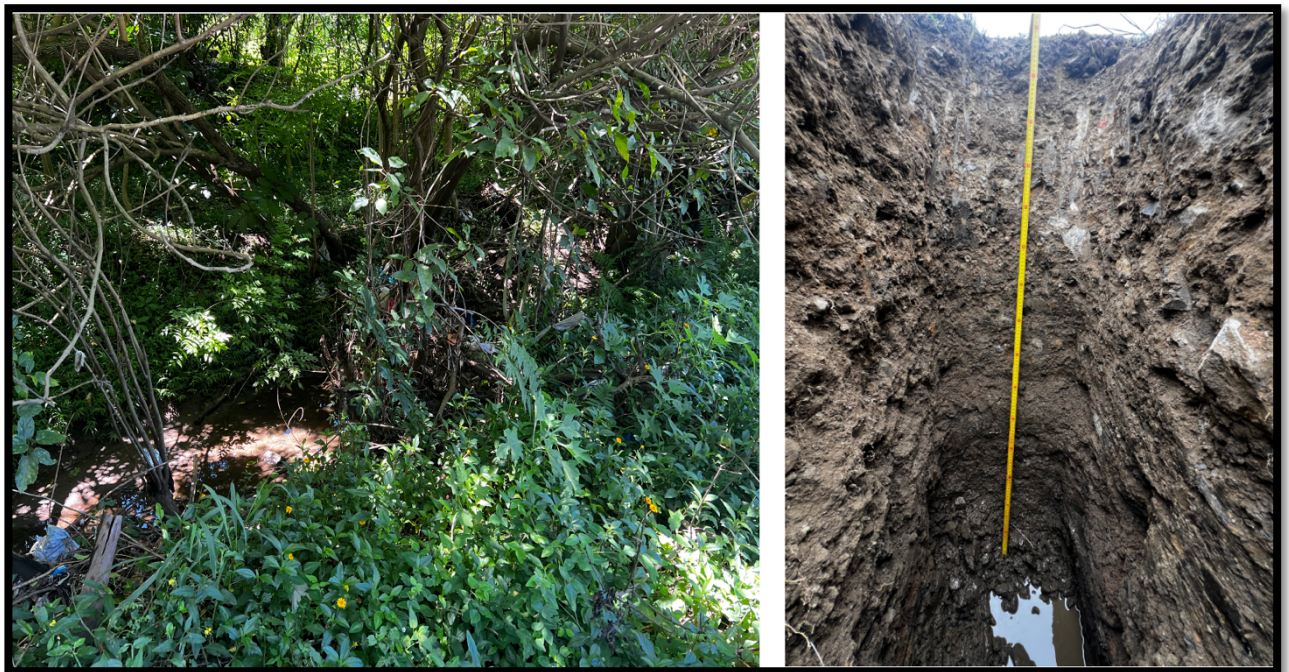
Figure 11: Showing the water in a stream intercepted along the pipeline as well as the groundwater seepage in a test pit.
