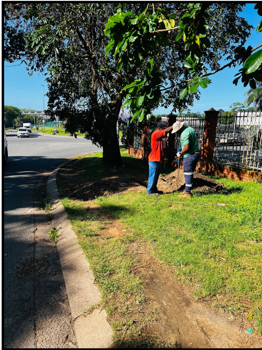
Figure 8: Showing the DCP testing undertaken at the site.
