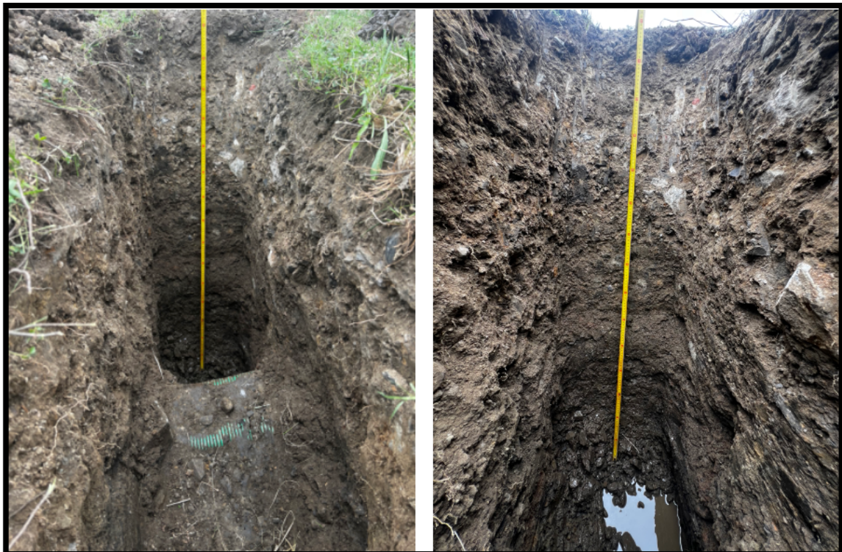
Figure 9: Showing the exposed cables inside the test pit and underground water seepage conservatively.
