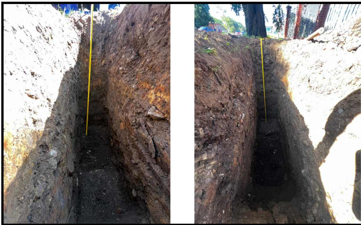
Figure 10: showing the stable test pit walls excavated at the site.
