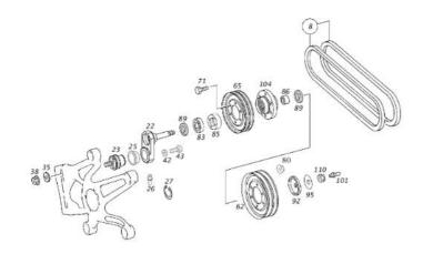
Guide Pulley Assembly - MA 4572004770
