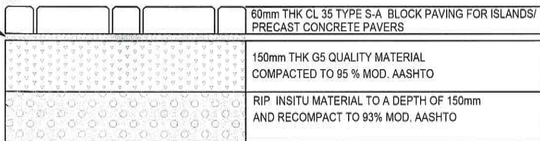
TYPICAL BRICK PAVING/ PRECAST CONCTETE PAVING LAYERWORK DETAILS N.T.S
