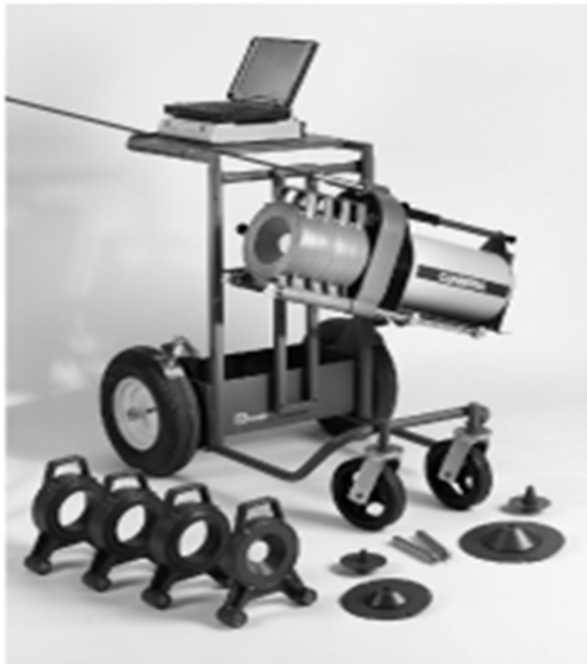
The ISOCS Detector, Cart, and Shield Components.
