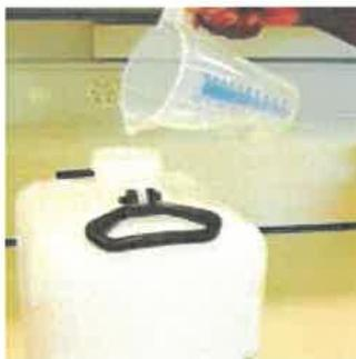
4. The bottle/tank is then topped up to the 10-litre mark with sterile distilled or cold boiled water.
