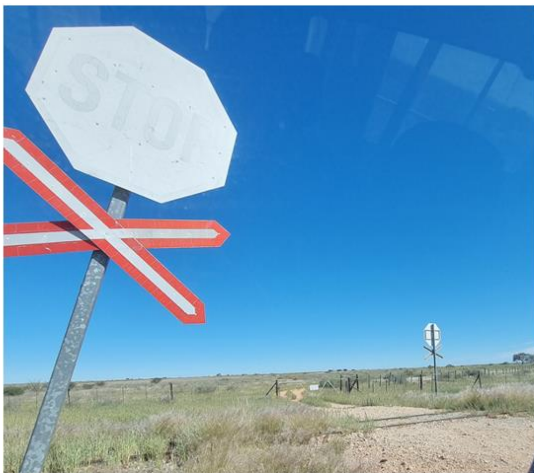
Figure 27: Faded and skew stop sign at km 13
