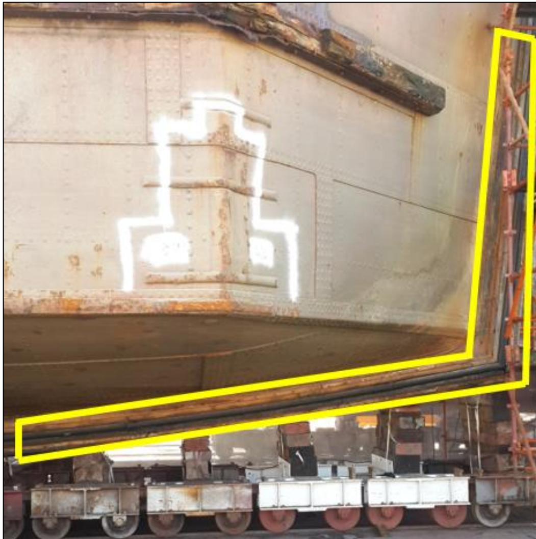
Figure 8: Yellow outline showing existing sealing face installation
