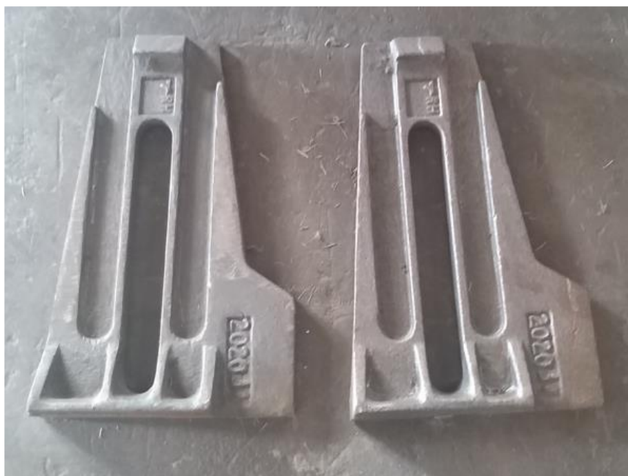
Figure 5: Illustrates the expected outlook for front stop castings post grinding and dressing.
