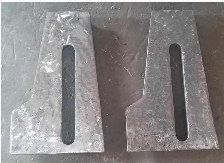
Figure 4: Illustrates the expected front stop outlook post grinding and dressing.
