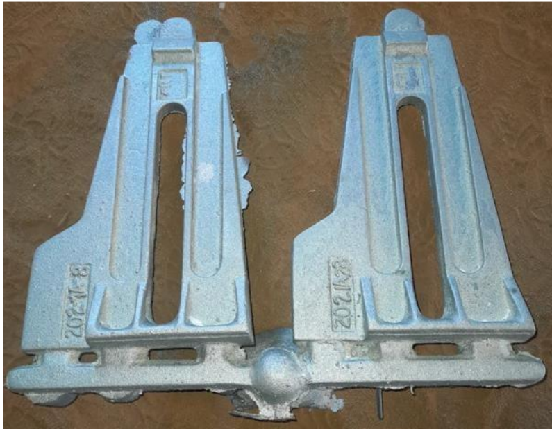
Figure 1: Bottom view of typical Front stop casting set, as received by supplier.
