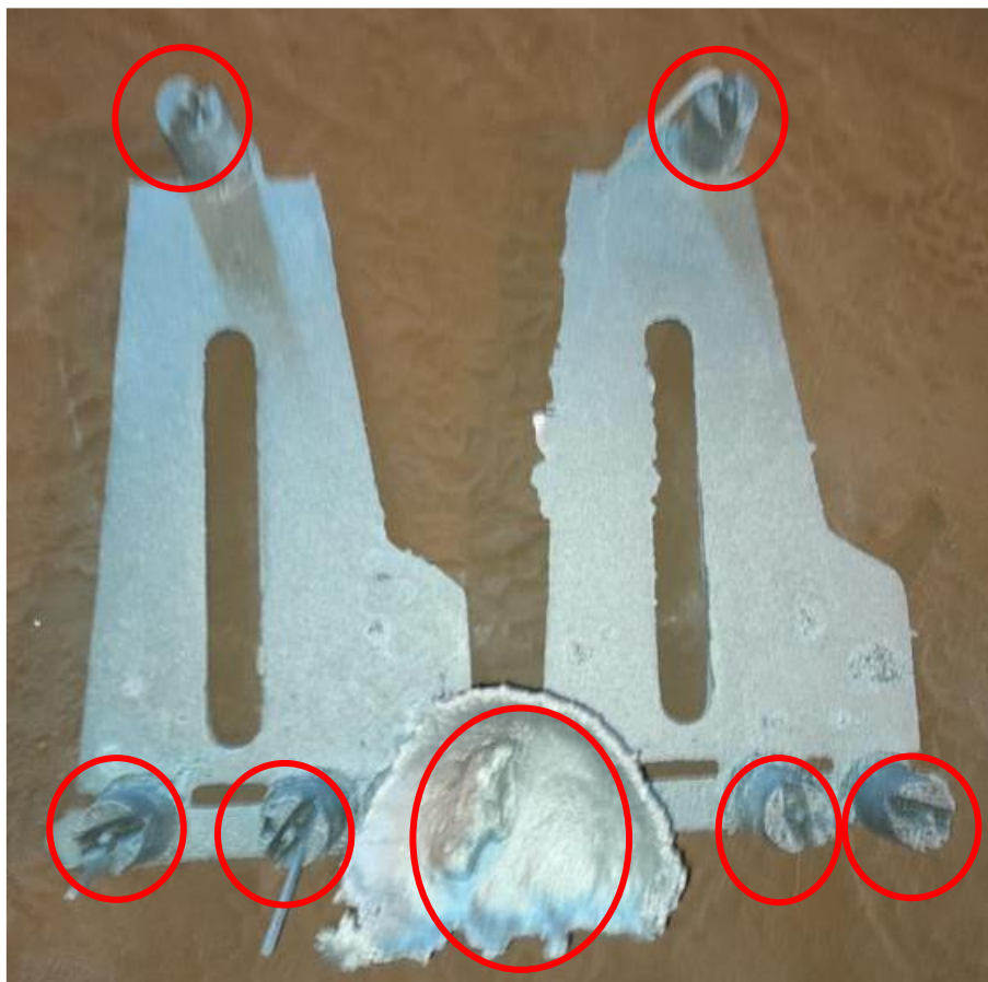
Figure 3: Illustrates relevant sections to be cut off. (NB: Removal of flesh is necessary)
