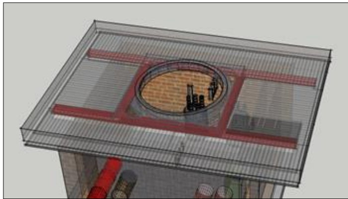
Fig. 18 The frame attached to the I beams
