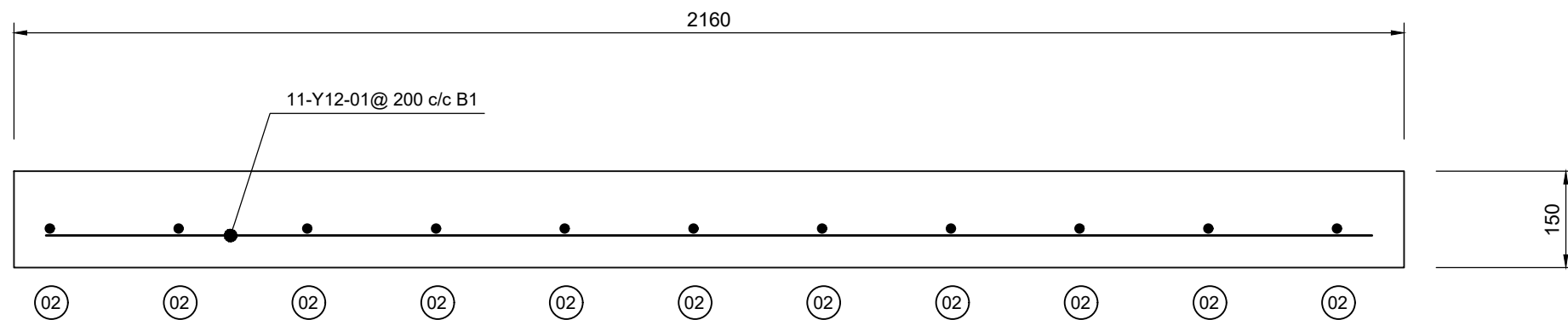
SECTIONAL VIEW OF REINFORCING DETAIL OF CONCRETE FLOOR SLAB SCALE 1:10
