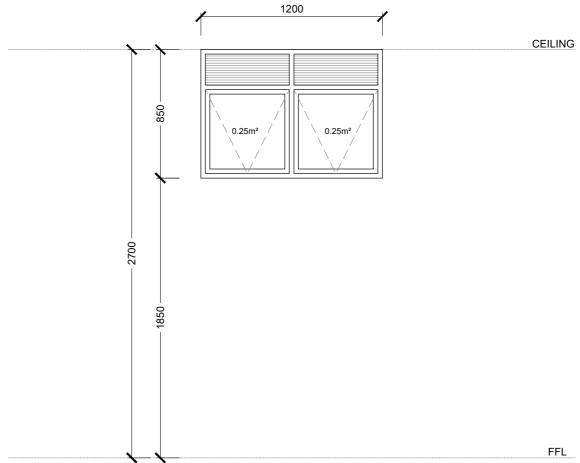
Type. R Crealco Swift 38 or eq. approved top hung aluminium casement window, per layout. Casement sash 1500 x 1200mm max capacity
